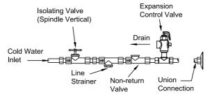
Note: a combined isolating valve/non-return valve/line strainer may be used.
